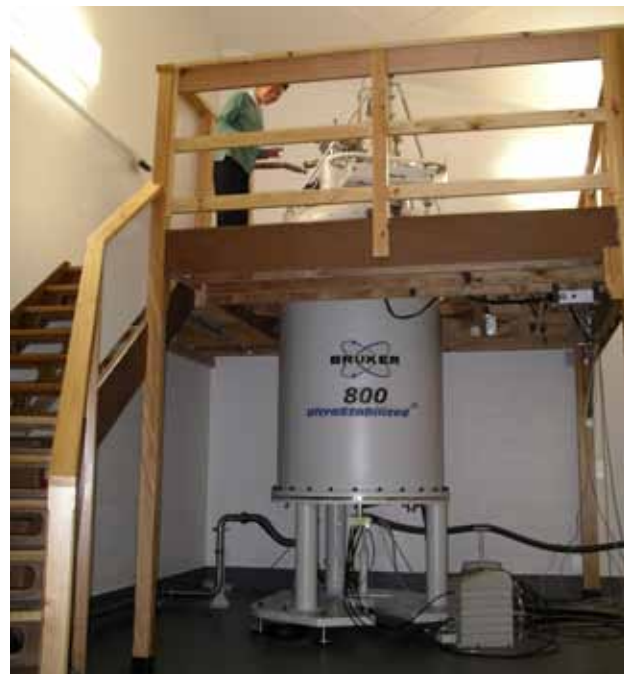
The 800 MHz magnet is one of Australia's highest field NMR systems.
