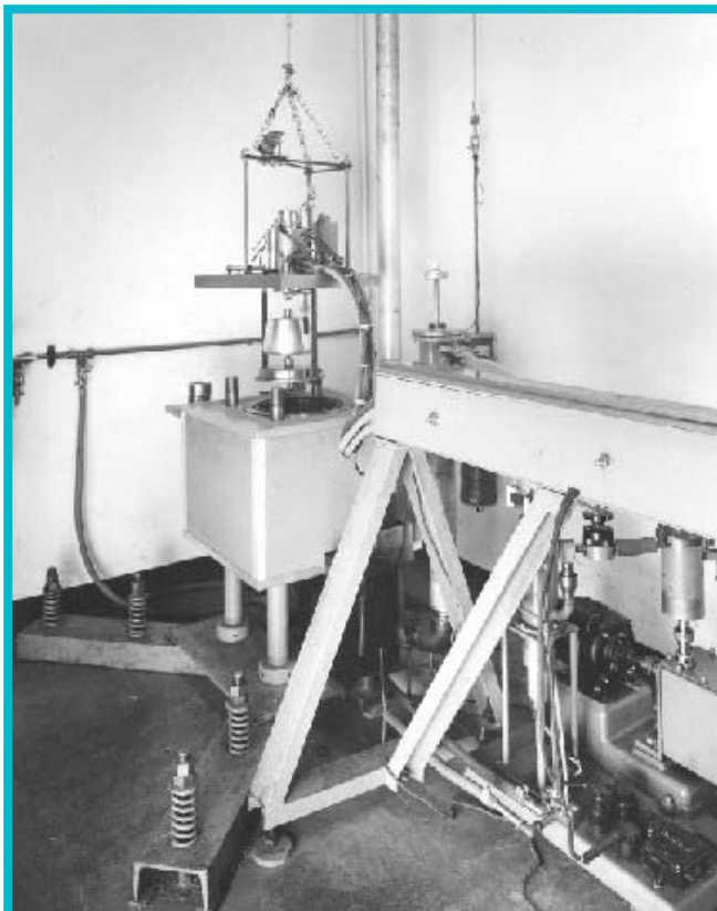
The Walter and Eliza Hall Institute air turbine analytical ultracentrifuge, showing the massive safety chamber with the rotor suspended by its thin wire shaft. Image from author's collection.
