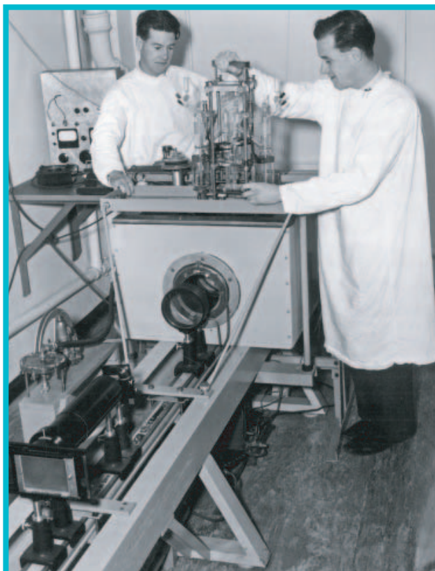
The Tiselius moving boundary electrophoresis apparatus built at the Walter and Eliza Hall Institute, with Gordon Ada left and John Pye right. The schlieren optical system and cells came from Adam Hilger, London. The rest of the instrument was sourced locally. Image courtesy of WEHI Archives.
