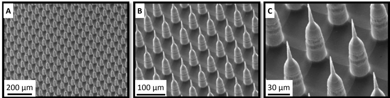
**Fig. 2.** The Nanopatch, a needle-free vaccine delivery system, magnified under scanning electron microscopy at **A.** 200-fold, **B.** 500-fold and **C.** 1200-fold magnification. These images show the individual projections of the Nanopatch, arranged in an ultra-high density array ( $>20,000$  projections/cm<sup>2</sup>), with high aspect ratio and tips with sub- $\mu\text{m}$  sharpness (15).
